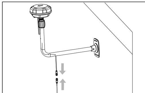
8. Connect the RTK reference station cable (10 m/33 ft.) to the RTK reference station power supply.
