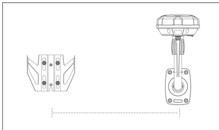
2. Drill 10mm/0.4 in. diameter, 35mm/1.4 in. depth holes.
