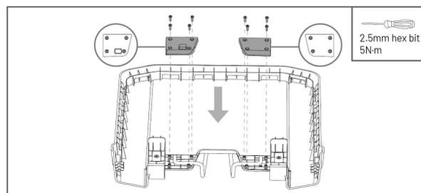
7. Embed the hopper into the hopper cover securely and gently pull both ends to adjust alignment.
