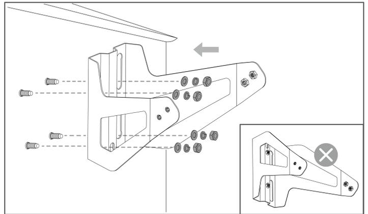
5. Secure the solar panel to the bracket with four screws and tighten using a 4mm/1.5 in. Allen key.
