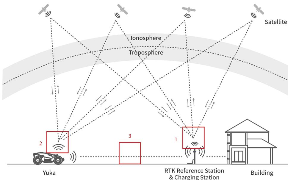
1. To perform its work, the RTK reference station receives satellite signals, requiring an obstruction-free environment and open-sky view.
