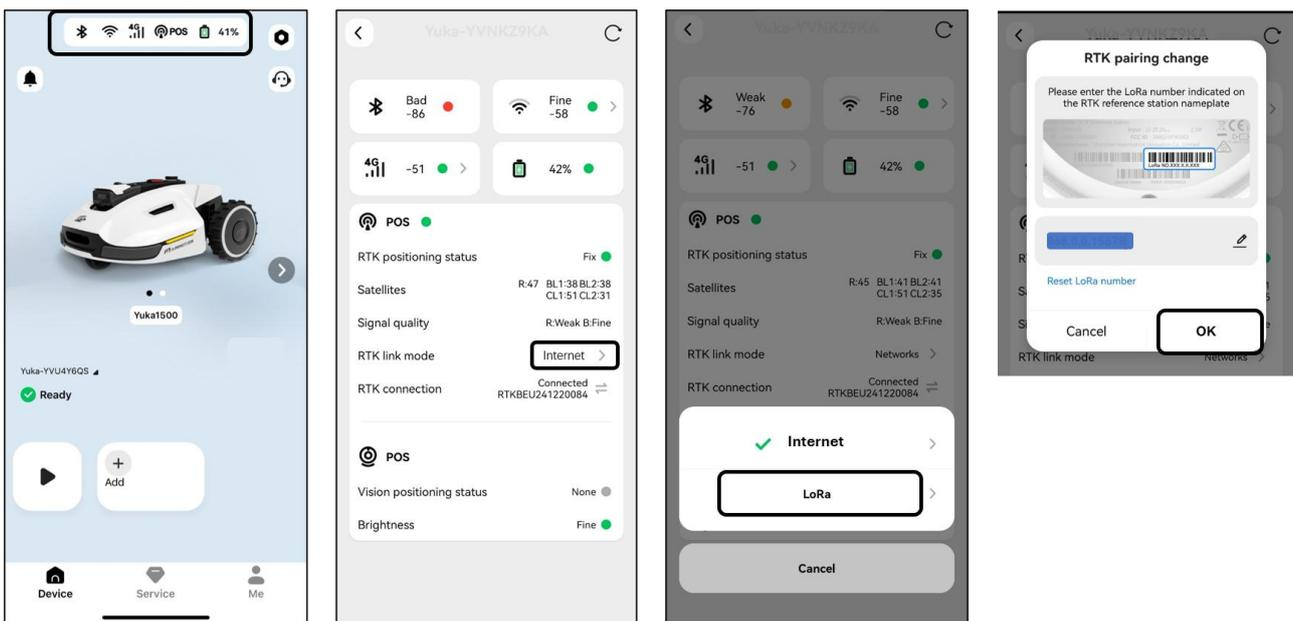
3. Return to the status information page and verify that the RTK link mode displays '**LoRa**', the RTK positioning status shows '**Fix**', and the RTK connection status shows '**Connected**'. Your setup is now complete.
