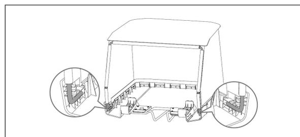
10. Assemble the sweeping brush module with the hopper module.
