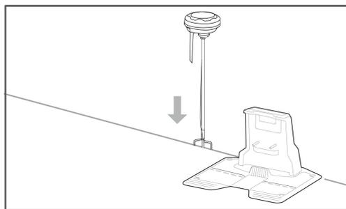
5. Thrust the mounting pole into the ground close to the charging station.
