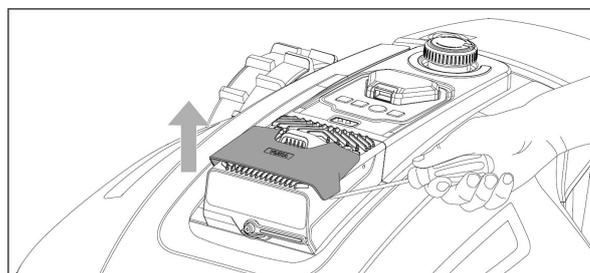
**15.** Attach the counterweight part onto the vision module.
