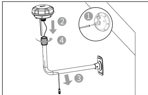
7. Connect the RTK reference station plug to the RTK reference station extension cable (10 m/33 ft.).
