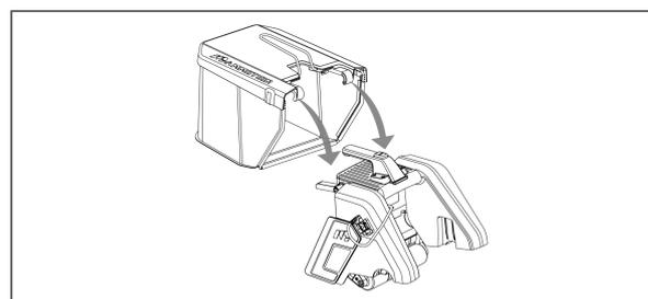
**11.** Insert the protrusion on the lawn sweeper into the slot on the rear of Yuka.
