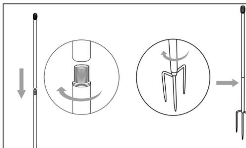
2. Fix the radio antenna to the RTK reference station.
