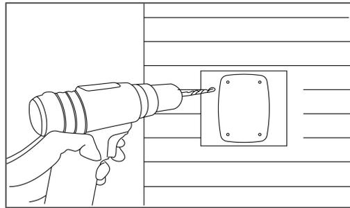
3. Attach the RTK wall mount on the wall using the four bolts (M8 x 50) and secure the bolts firmly.
