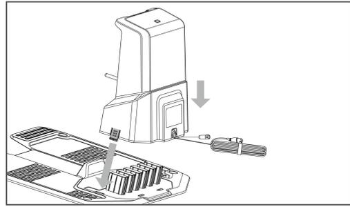
2. Install and tighten the three screws from the bottom of the charging base plate using the screwdriver with the 2.5mm hex bit.
