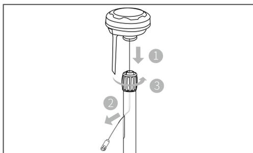
4. Mount the RTK reference station on the mounting pole.
