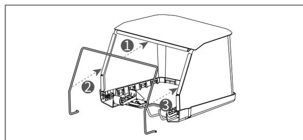
9. Securely insert both ends of the U-shaped support rod into their designated positions.
