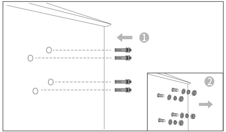
4. Attach the bracket to the wall without reversing it. Reinsert washers, spring washers, nuts, and tighten with a 13mm/0.5 in. socket wrench.
