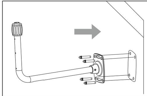
4. Fix the radio antenna to the RTK reference station.
