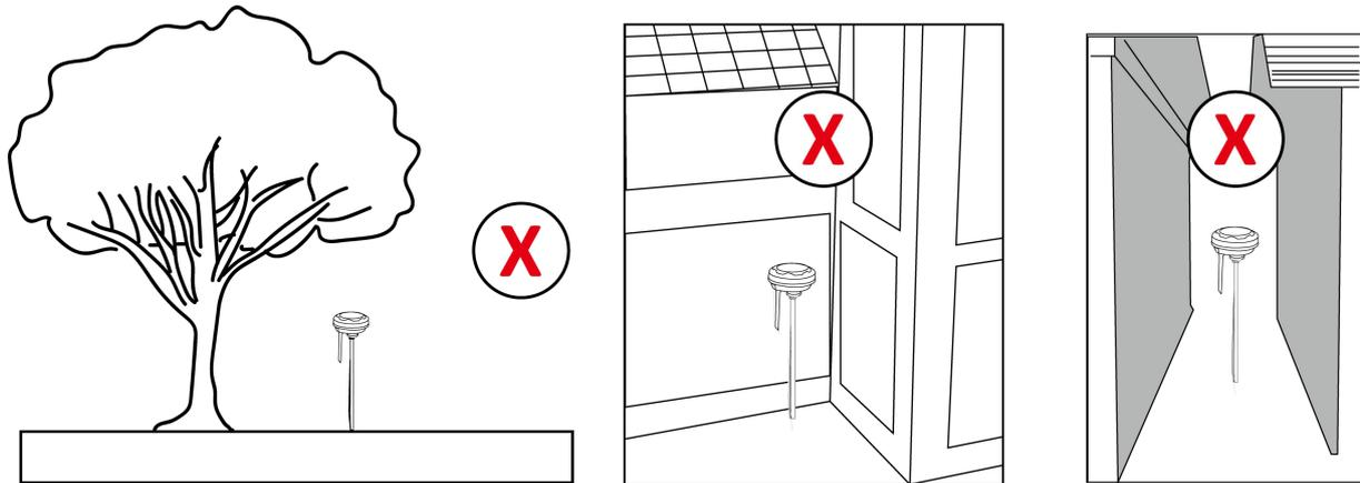
If you need to install an RTK solar panel kit, for optimal exposure to sunlight, Mammotion recommends the following locating guidelines:
