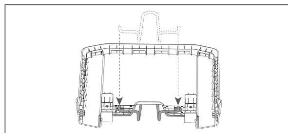
6. Attach the two hold-down plates to secure the hopper handle in place. Tighten the 8 screws using the screwdriver with the 2.5mm hex bit. Note that the torque should not be over 5 N·m.
