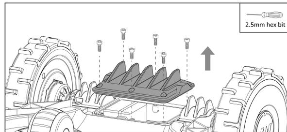
2. Connect the battery wires and use the two screws to secure the battery. Tighten the screws using the screwdriver with the 2.5mm hex bit.
