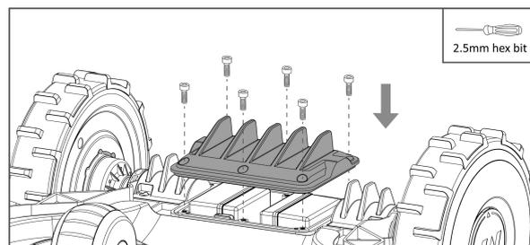
4. Install the handle module on top of the sweeping brush module and tighten the 4 screws using the screwdriver with the 2.5mm hex bit.
