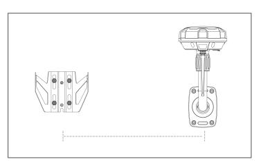
Drill 10mm/0.4 in. diameter, 35mm/1.4 in. depth holes.
