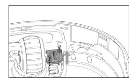
Eject the SIM card tray using the SIM-eject tool, install the SIM card, and push the card tray into place.
