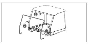
Securely insert both ends of the U-shaped support rod into their designated positions.
