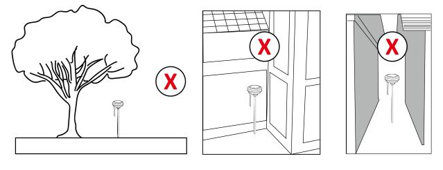
If you need to install an RTK solar panel kit, for optimal exposure to sunlight, Mammotion recommends the following locating guidelines:
