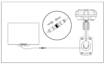
**7.** Connect the solar panel cable to the RTK reference station cable.
