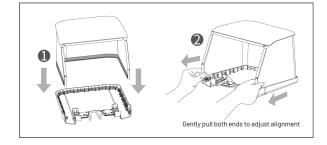
Insert the U-shaped supporting rod into the hopper.
