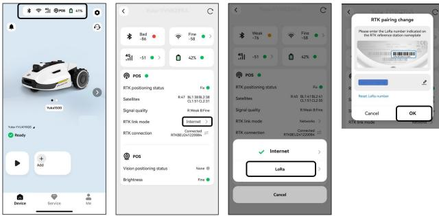
Return to the status information page and verify that the RTK link mode displays 'LoRa', the RTK positioning status shows 'Fix', and the RTK connection status shows 'Connected'. Your setup is now complete.
