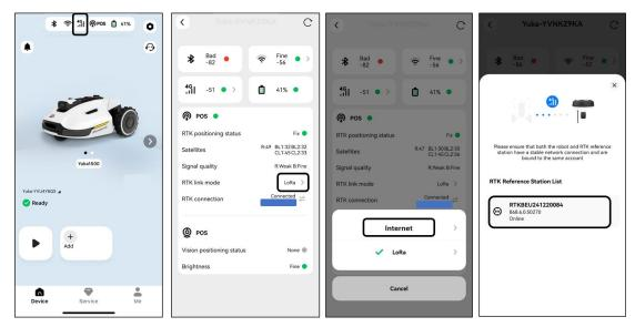
**3.** Wait for a green check mark to appear, then return to the status information page. Verify that the RTK positioning status displays '**Fix**' and the RTK connection shows '**Connected**'. Your setup is now complete.
